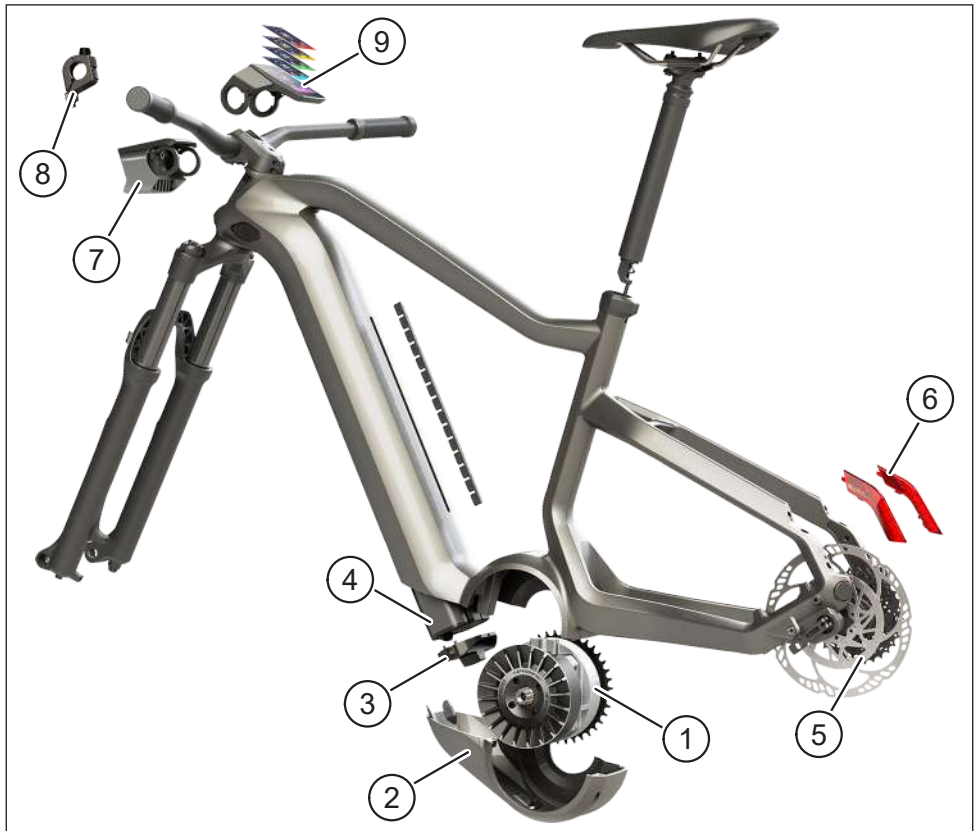
Fig. 1: Components of the FLYON drive system
